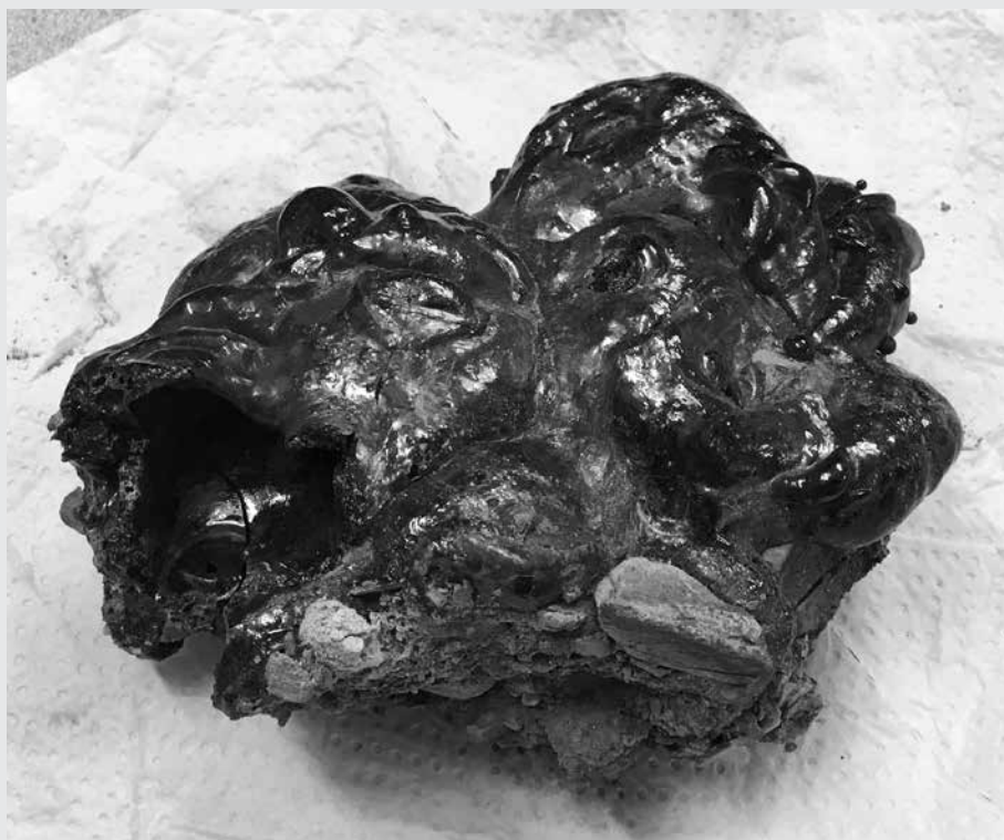
A cautionary image courtesy of WEC Director of Products and Services Bill Powell. This molten space rock was created when a downed power line touched driveway gravel. Imagine what that same voltage could do to you. Never go near a downed wire!
